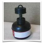
The second type of measurement devices are called electret ion chambers. This device consists of a special plastic canister (ion chamber) containing an electrostatically charged disk detector (electret). The detector is exposed to radon in the air during the measurement period. Ionization resulting from the decay of radon produces a reduction in the charge on the electret. The drop in voltage on the electret is related to the radon concentration.
